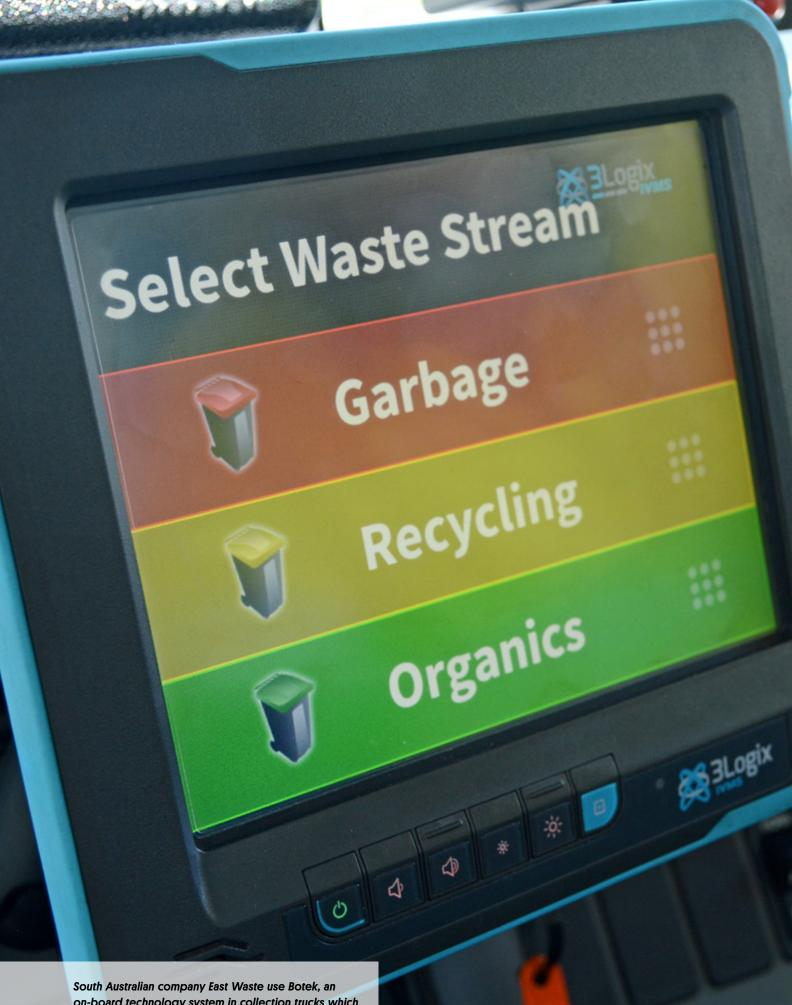
South Australian company East Waste use Botek, an on-board technology system in collection trucks which provides real time data for the kerbside-collected three bin system
